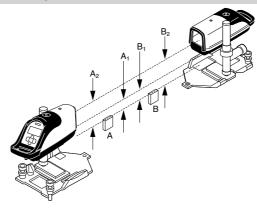
Checking the calibration of your pipe laser is simple with an engineer's rule and your pipe laser.
